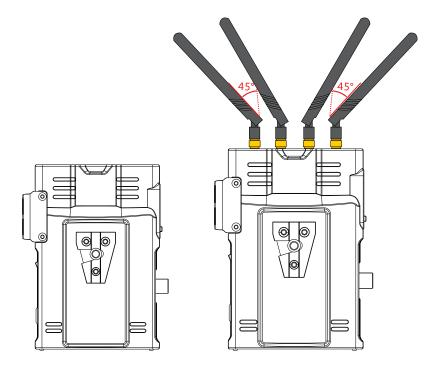
2. Please fix the transmitter via the screw at the bottom or the V-mount at the back, and place it at a height of around 1.5 to 2 meters above floor. Please make sure that the distance between each transmitter is more than 1 meter.
