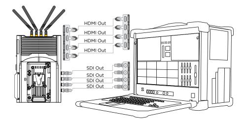
4. The receiver can be powered by both the V-mount battery and DC-IN port via the affiliated power adapter. If the mentioned two types of power supply are connected at the same time, the lithium battery is prioritized in power supplying, and the battery will switch to the power adapter for power supplying automatically after the battery power is exhausted.
