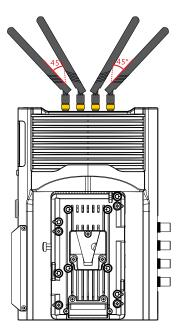
2. Please place the receiver at a height of around 1.5 to 2 meters above floor. Receiver can be placed in vertical or horizontal positions, and can be fixed via the screw at the bottom or V-mount at the back. Please install the affiliated metal stand before placing the receiver in vertical position.
